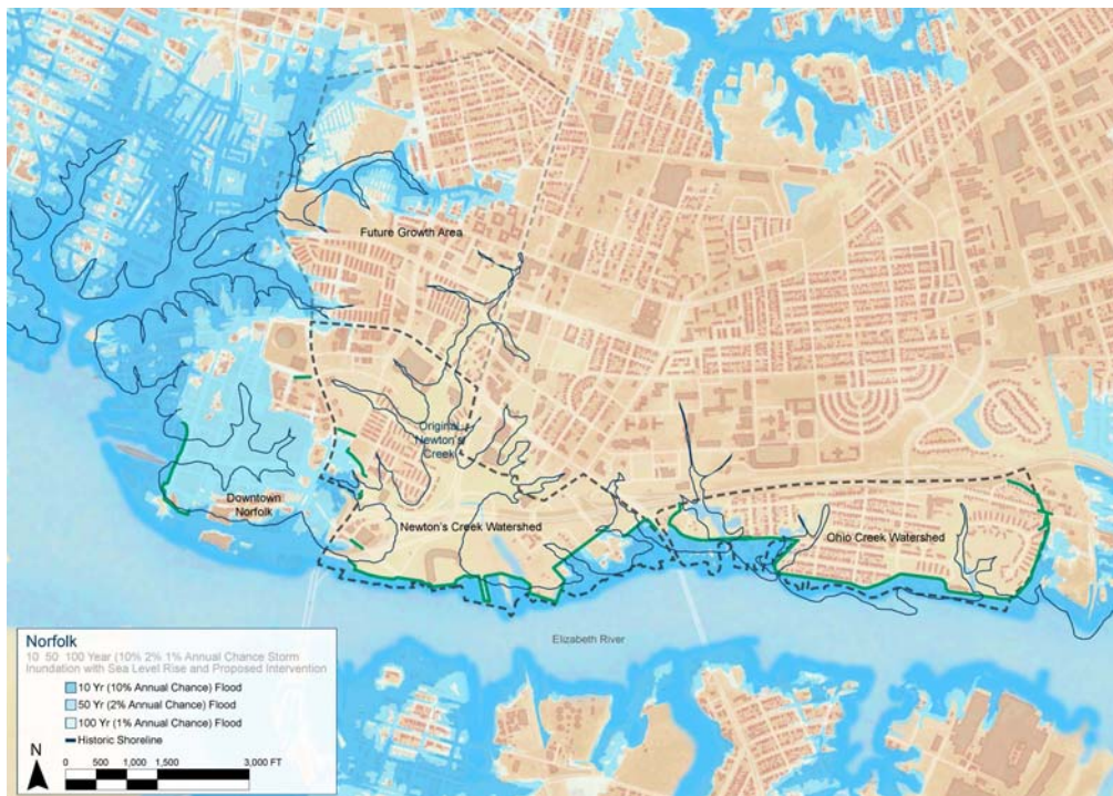
Figure IV.1.1.6 Estimated Flood Extent of 1% Annual Chance Given 2.5 Feet of SLR and Proposed Improvements
