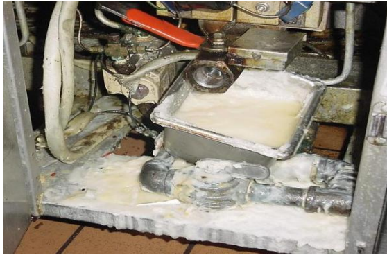
Grease leaking out of a faulty valve under a deep fryer
