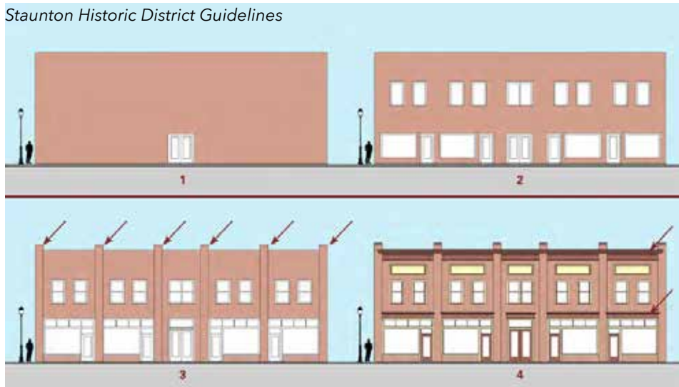
This illustrations shows how architectural elements and details bring buildings into relationship with the human scale.
