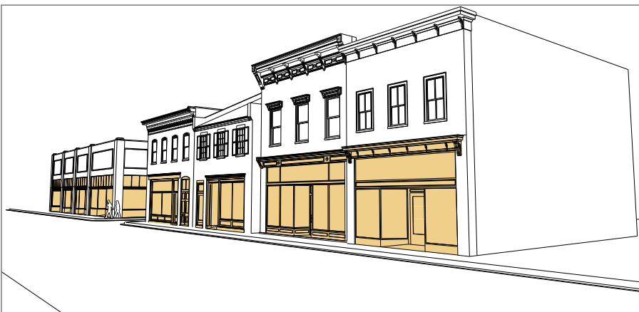
The first floor is typically transparent storefronts.
