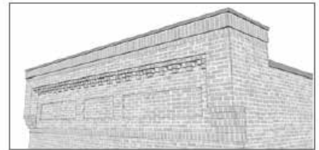
Sample brick cornice
