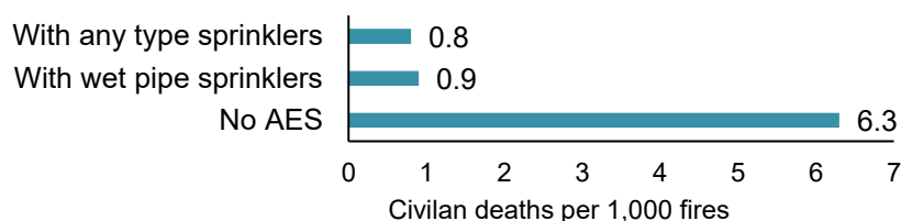
Figure 4. Civilian death rates per 1,000 fires in properties with sprinklers and with no AES: 2010-2014
