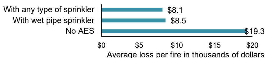
Figure 22. Average loss per fire in homes with sprinklers and with no AES 2010-2014
