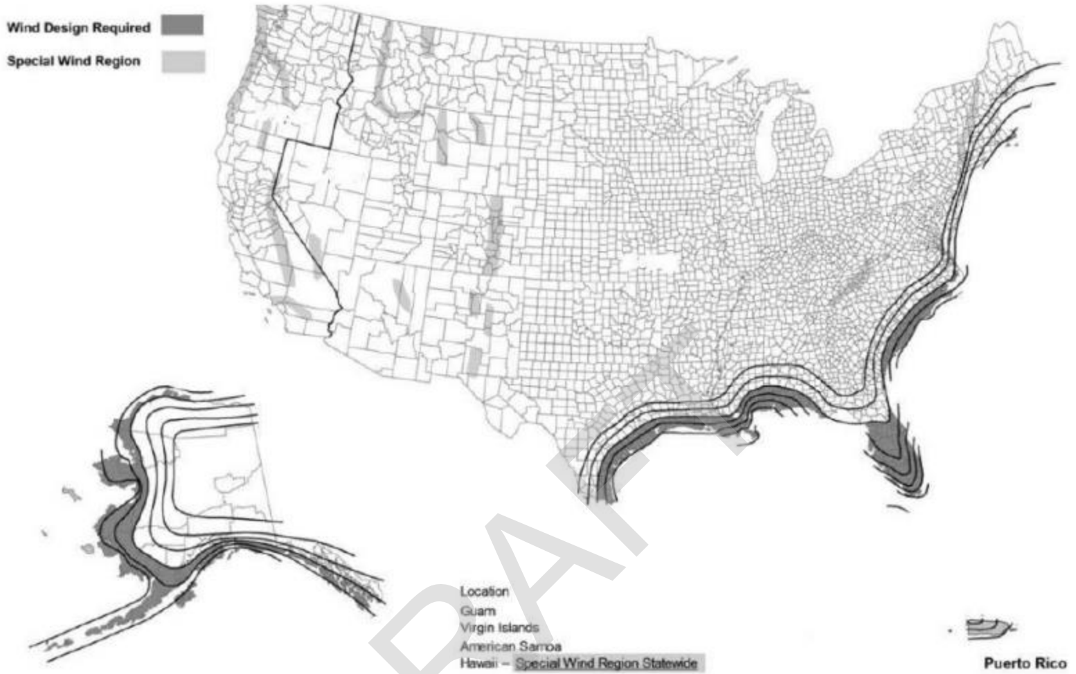
Figure R301.2(5)B REGIONS WHERE WIND DESIGN IS REQUIRED 9. Change Figure R301.2(8) to read:
